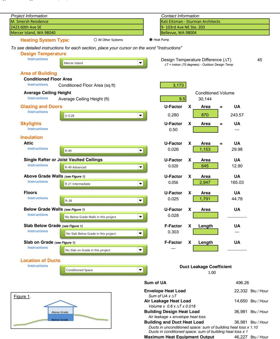
Building and duct heat loss x 1.40 for forced air furnace Building and duct heat loss x 1.25 for heat pump
